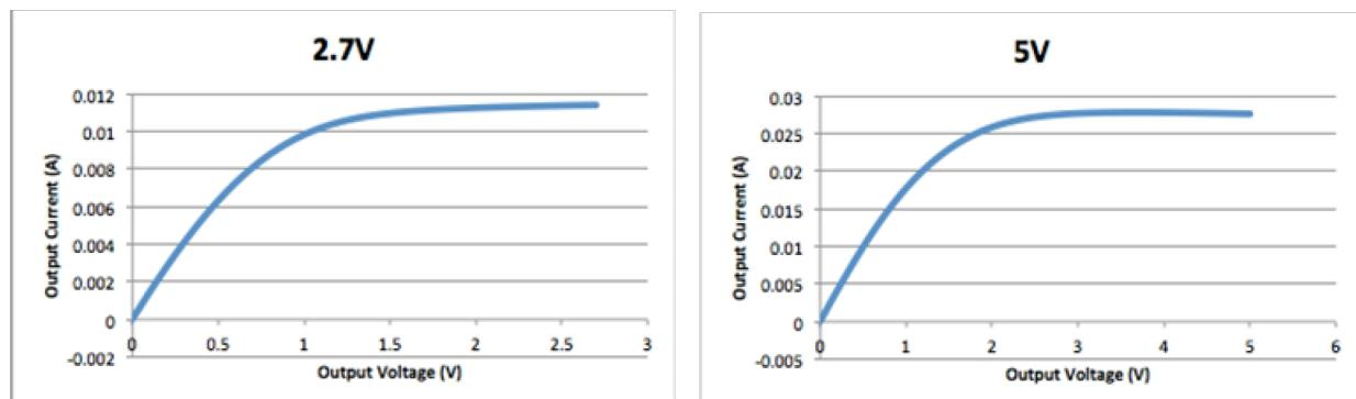
**Output Voltage vs. Output Current Sink Sweep**
